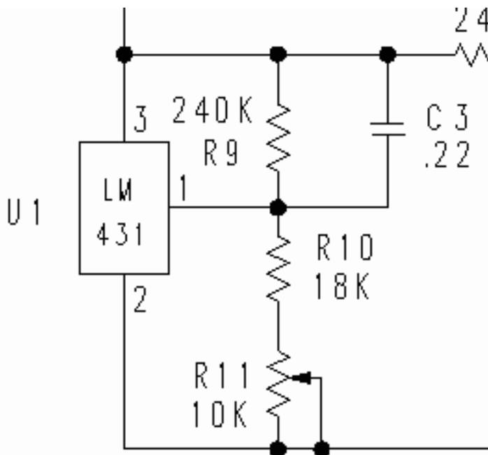
When I refer to the voltage reference this is the part of the circuit I'm referring to.
