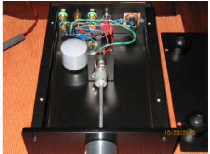
A closer look shows the optocouplers mounted very close to the connectors; Wiring looks more than necessary because of my decision to have 2 pairs of outputs and switchability to headphones:
