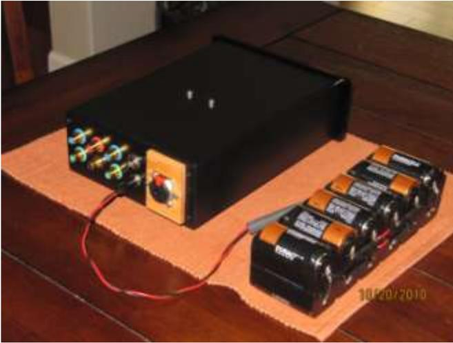
A closer look shows the back panel sporting a pair of inputs; 2 pairs of outputs; a power, line or headphones switch; power input plug; and a headphones out:
