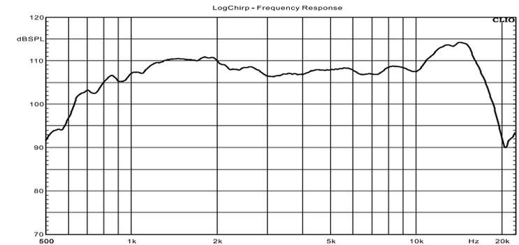
Test conditions: 1W/1m standard test box in anechoic chamber.
