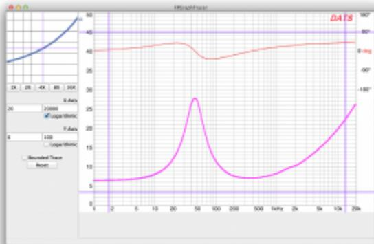
Step 3: The 4 purple bars will need to be adjusted so that accurate data can be extracted from the sampled points. Place them over known axis values. To achieve the highest level of accuracy, they should be placed far apart and the zoom window used to place them precisely.
