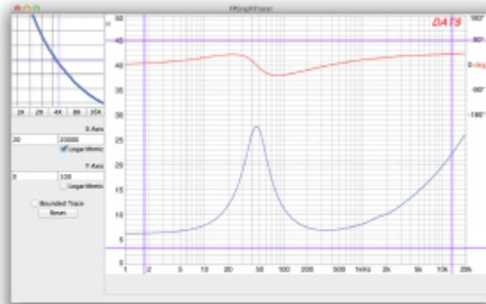
FPGraphTracer is a simple, easy to use, tool for automatically tracing lines in a graph to extract the data it represents. Originally intended for the DIY speaker community, it outputs in the FRD/ZMA text based format used by many speaker designing programs, which can also be pasted directly into most Spreadsheet software.
