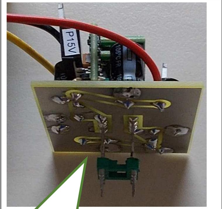
You cannot see on the picture but the pin 4 and 8 are connected to the green support
