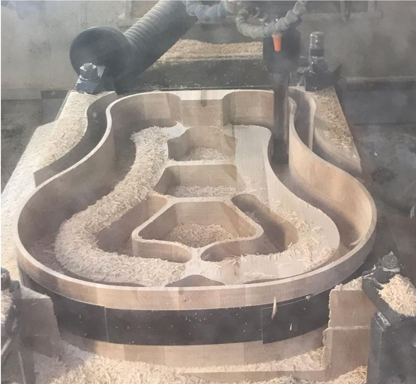
CNC machine almost complete. I can cut the entire body and horns in about two full days, runs at night.
