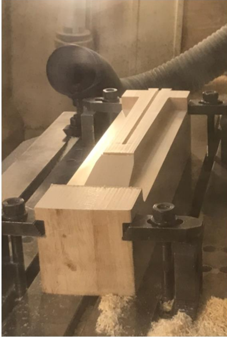
Solid stock on the CNC machine.
