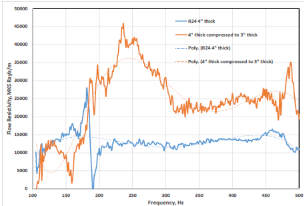
Figure 6.13 – Three microphone method: Flow resistivity of R24 4" sample [39]
