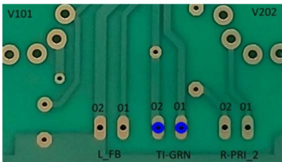
Measure at connector T1-GRN, pins 1 & 2 (blue circles), you should have 5.9 to 6.3 volts A.C. This is the 6.3V A.C. 4 Amp Heater supply.
