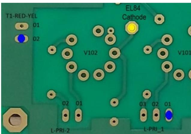
Measure the DC voltage at connector T1-RED-YEL, pin 2 and connector L-PRI\_1, pin 1 (blue circles), it should be around 320 volts.
