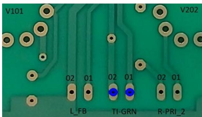
Measure the voltage at the connector T1-GRN, pins 1 & 2 (blue circles).
