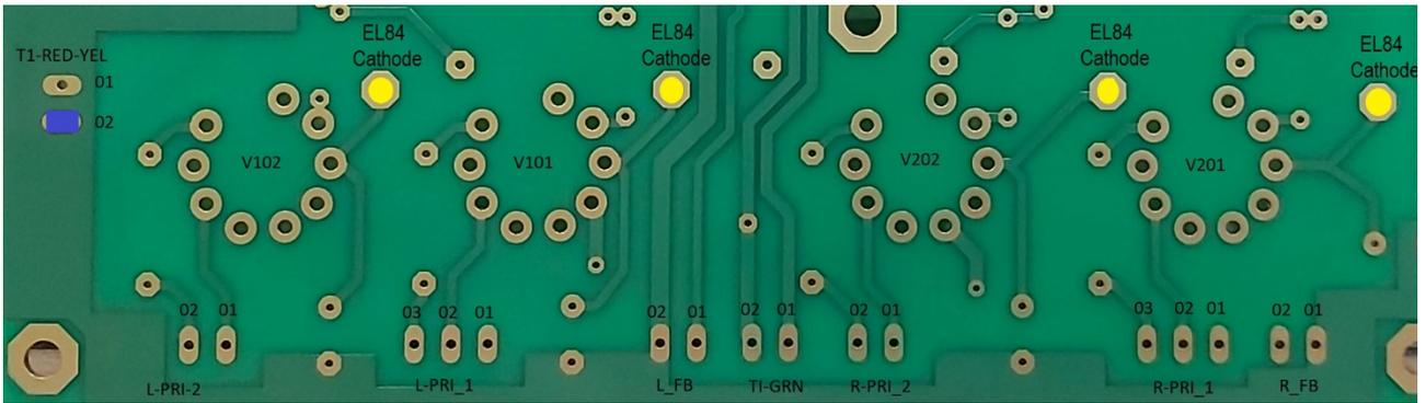
We now need to measure the D.C. voltage on each cathode of the four EL84 valves.
