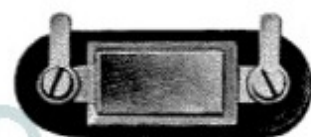
Internal View of Fixed Condenser
