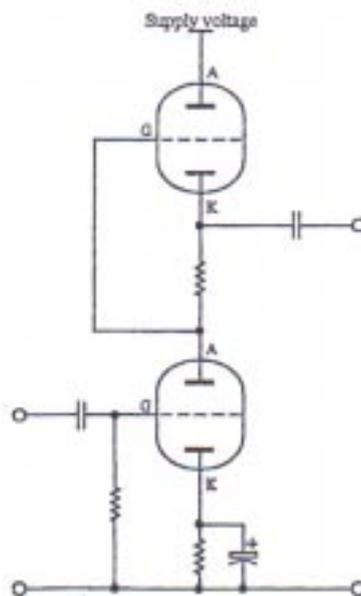
The lower valve is a normal cathode coupled amplifier as we already know it, but the anode load resistor is replaced with a valve coupled as a cathode-follower. The term cathode-follower has been used since Adam was a boy, but is in fact misleading because what really happens is that the cathode voltage is forced to follow the grid voltage so the term grid follower would be more
