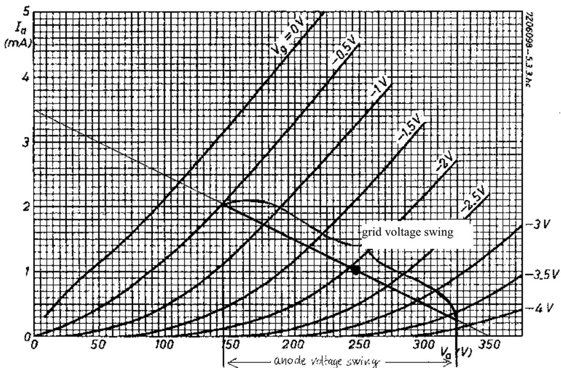
Again the working line is drawn for  $V_{\text{supply}} = 350V$
