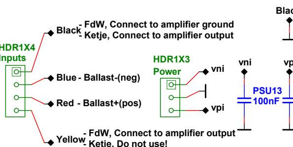
J1/2/3 Connect pin 1 to 2 on all 3 headers for method 'FdW' (full circuit).
