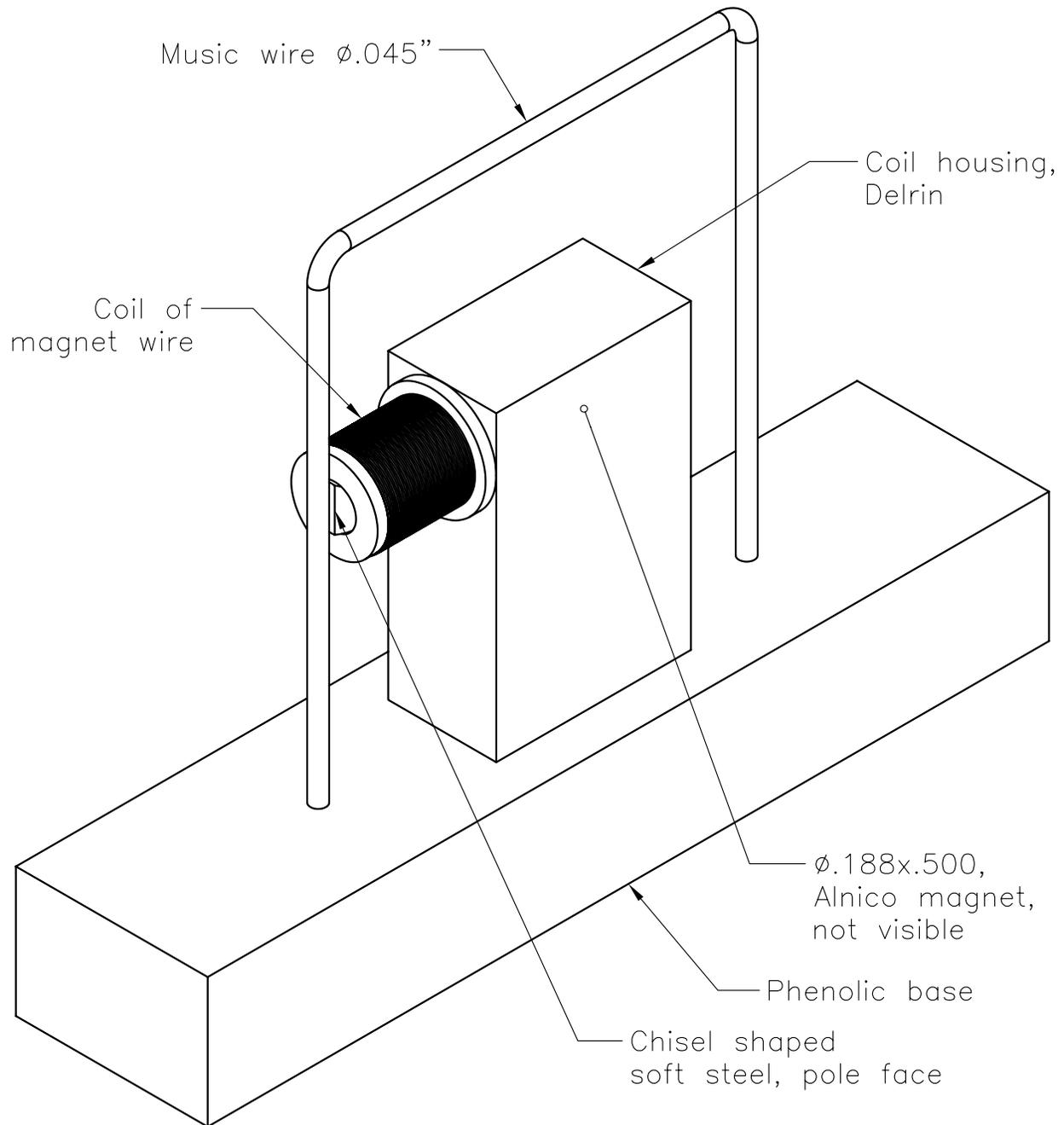
This is the first experimental picking switch assembly.
