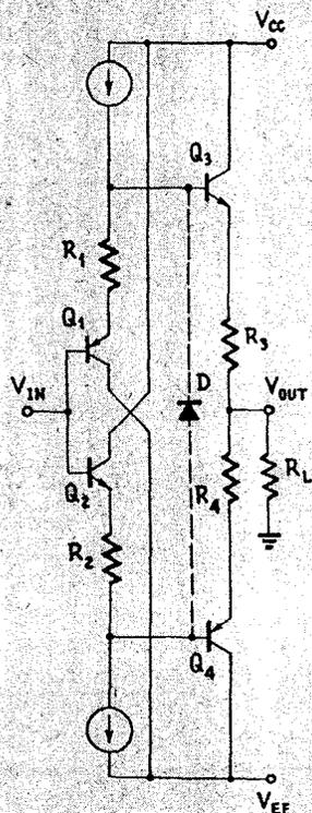
Fig. 1. The basic circuit of the unity-gain buffer.
