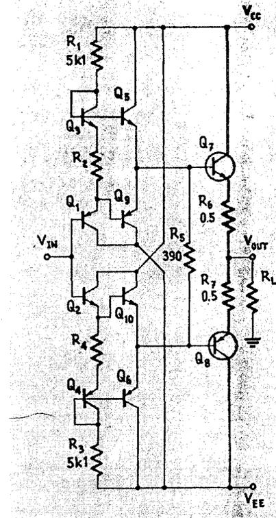
Fig. 5. Improved version of Fig. 4a circuit with additional emitter followers (Q<sub>7</sub>, Q<sub>8</sub>) for fast output transistor turn-off.
