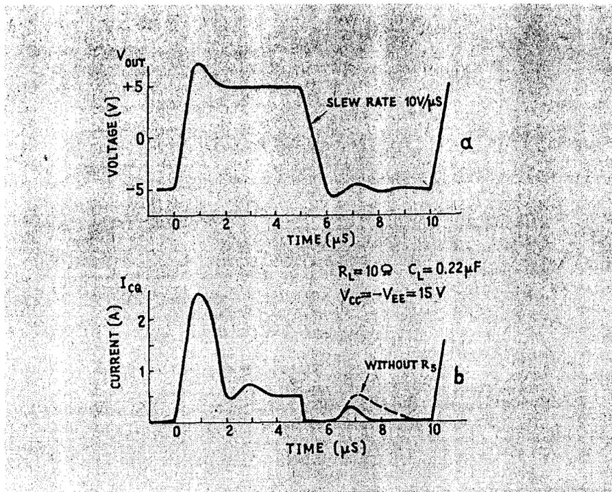
Fig. 7 Transient responses of Fig. 5 circuit driving a 10Ω load with 0.22μF in parallel, output voltage (a) and Q<sub>7</sub> collector current (b). Lower graph shows the effect of R<sub>5</sub> moving.
