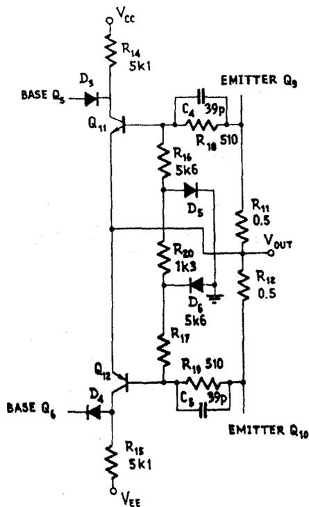
Fig.10. Suitable overload protection circuit with SOA control.
