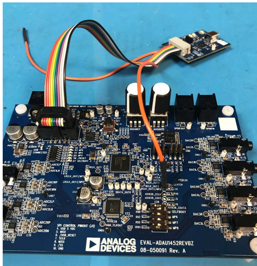
Figure 81. Completed Modification with EVAL-ADUSB2EBZ (USB) Connected.
