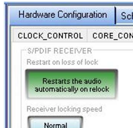
Figure 37. Activating the SPDIF_RESTART Register, Changed Button
