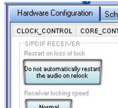
Figure 36. Activating the SPDIF_RESTART Register, Initial Button
