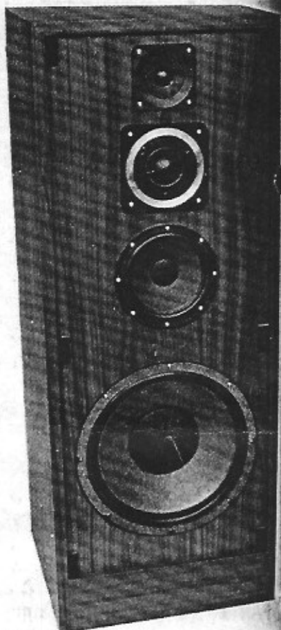
The 4000/1 loudspeaker, without the front grille, showing the drivers. It stands about one metre tall.
