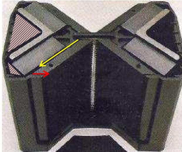
The cause is probably some of the sound emitted from the outer lateral regions of the membrane, which reaches the inner workings of the AMT-1. Unfortunately, you cannot open the chassis as shown in the picture, because then you should also insert absorption material in the outer areas (pink hatched area).
