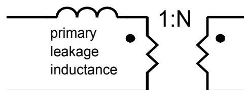
Figure 72 Leakage inductance at the primary side.
