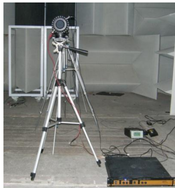
Figure 6: The test of frequency response of SPL of compression driver.
