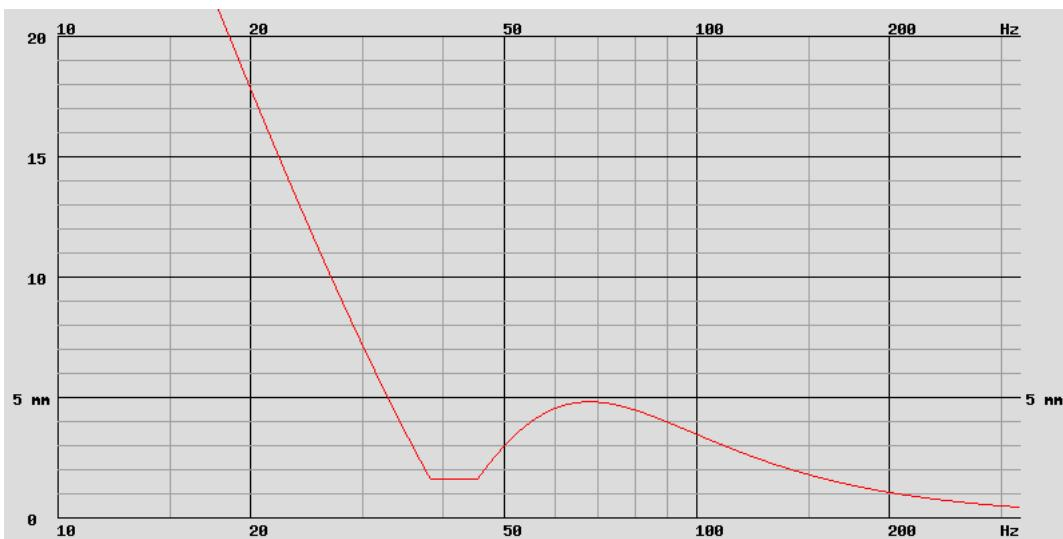
The flat around 41.6 Hz is not the strict reality of things. It is however fairer than a curve of displacement which passes by 0 to 41.6 Hz.
