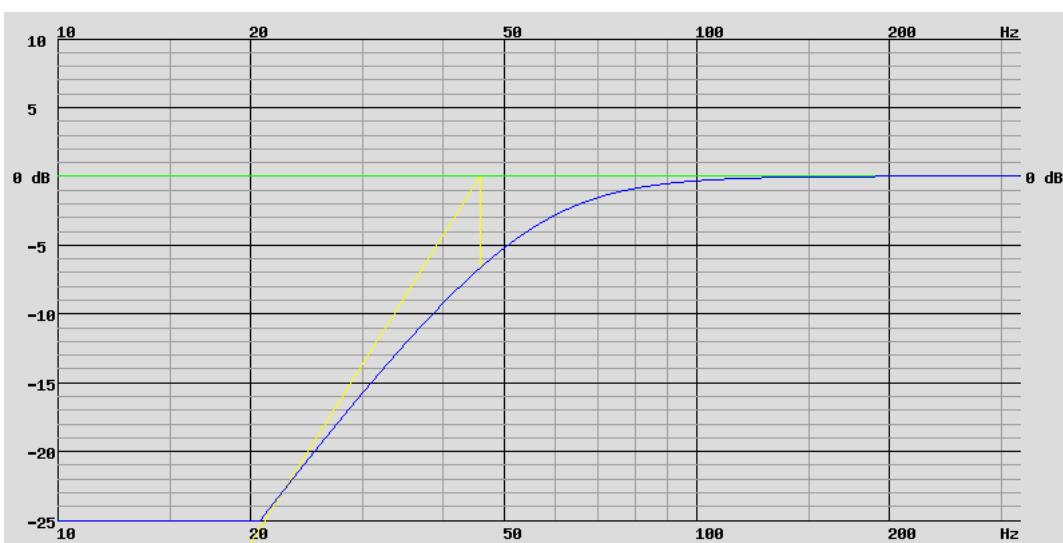
The response curve is calculated in [free field](#), outside on a mast 15 m high, far from any obstacle.
