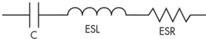
When the capacitor is connected across a signal line, its impedance will decrease with increasing frequency; the impedance will be at a minimum at resonance, rather than at some high frequency. At resonance, the impedance will be lower than the
