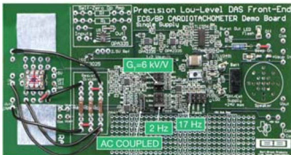
Figure 1 EMI from a cell phone can cause a 1.5V change from normal on an ECG. The ECG diagnostic tool senses a heart while a 0.5W, 470MHz transmitter turns on and off just one and a half feet away.
