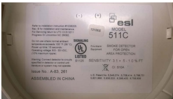
image 3 of 3 ESL, the date code and model are printed on a label on the back of the detector's cover.
