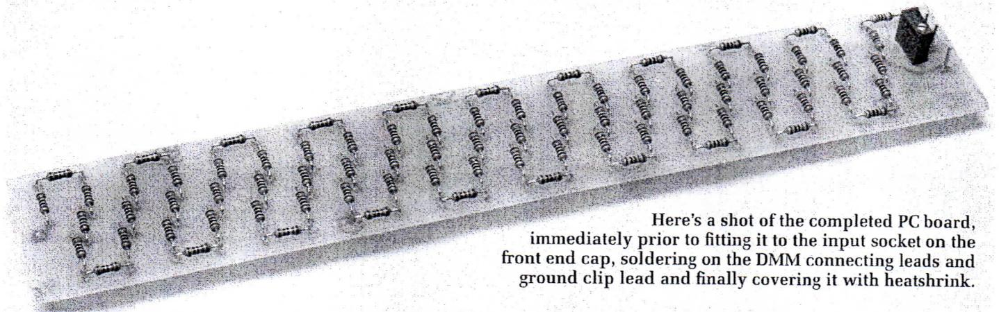
Here's a shot of the completed PC board, immediately prior to fitting it to the input socket on the front end cap, soldering on the DMM connecting leads and ground clip lead and finally covering it with heatshrink.
