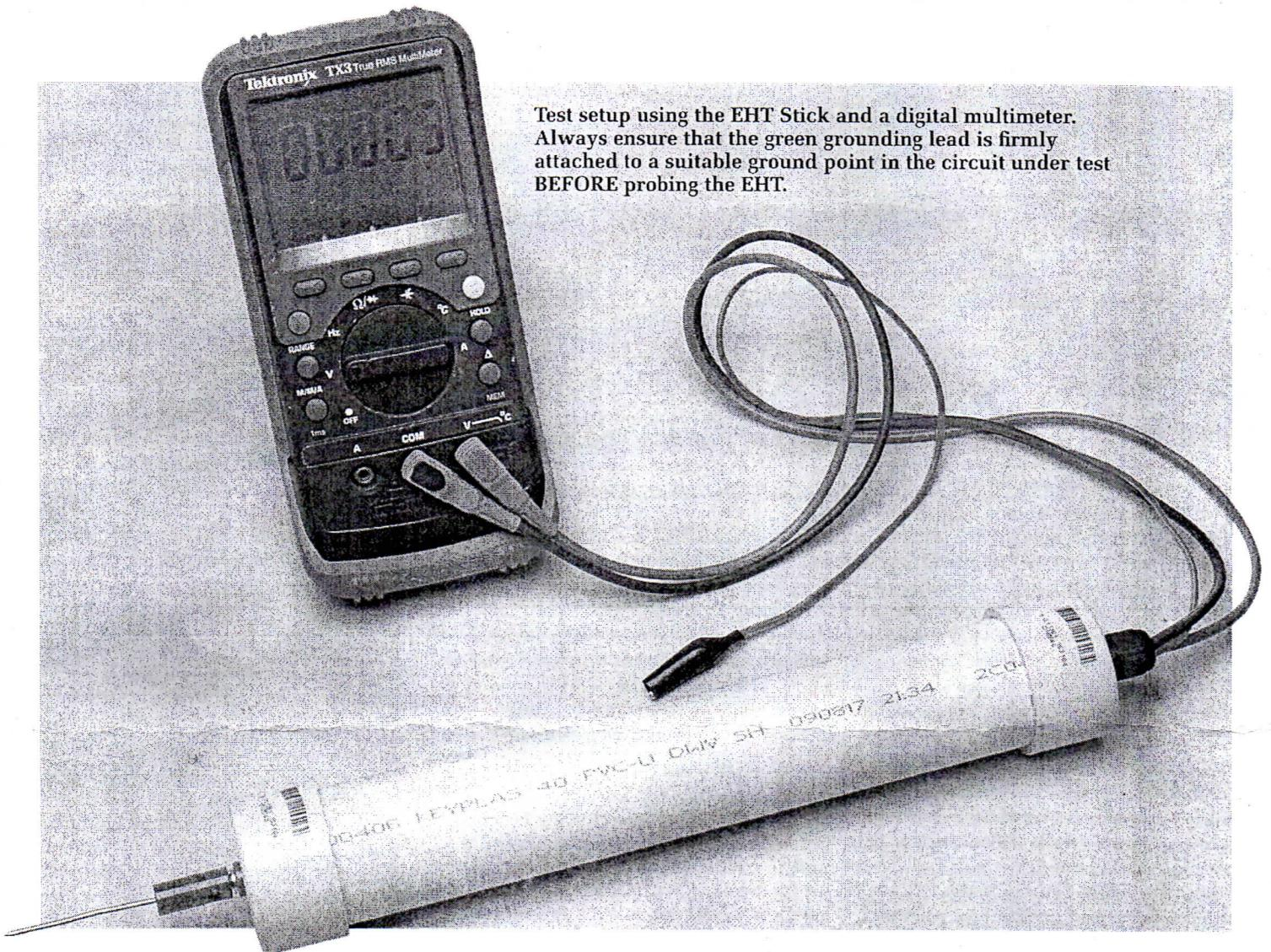
Test setup using the EHT Stick and a digital multimeter. Always ensure that the green grounding lead is firmly attached to a suitable ground point in the circuit under test **BEFORE** probing the EHT.
