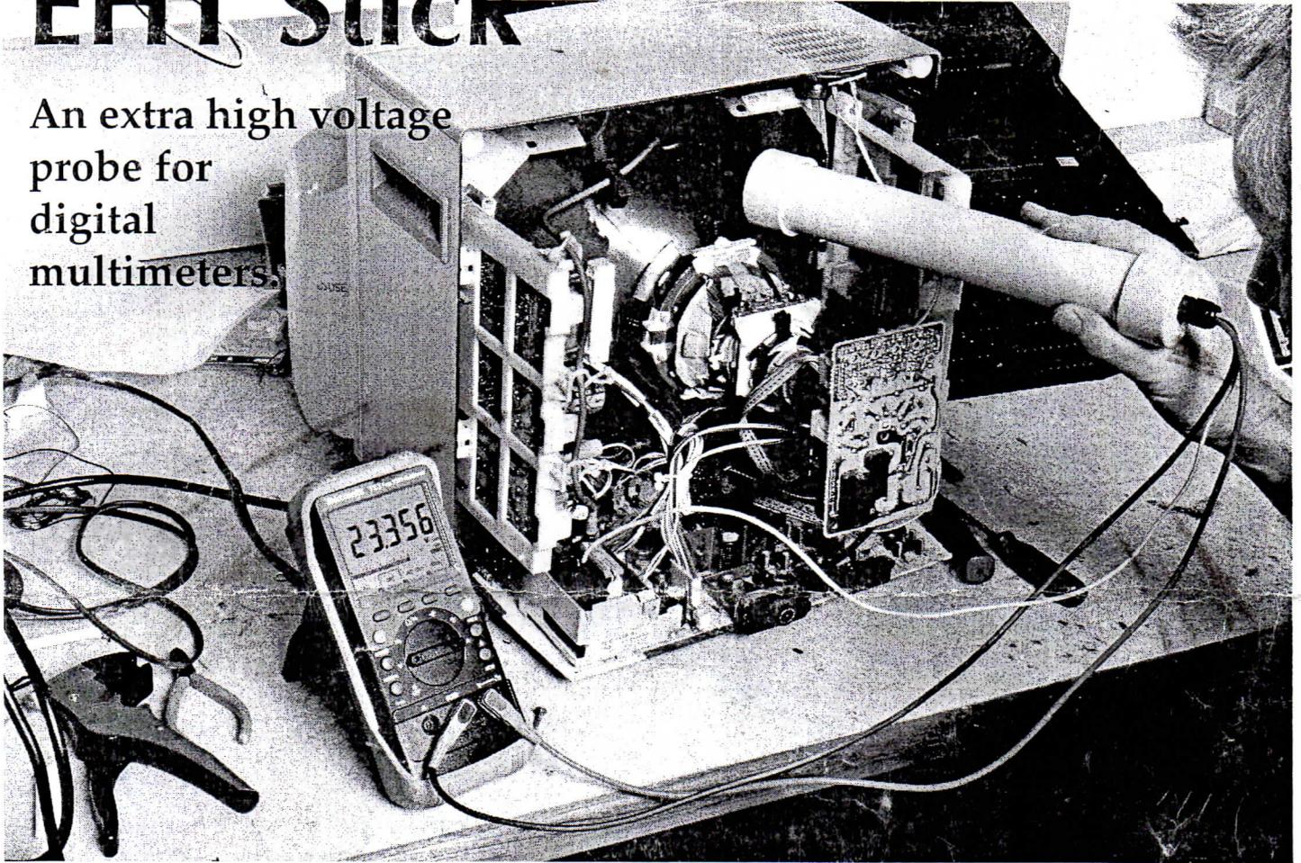
Do you need to measure the EHT voltage in a CRT-based scope, computer monitor or TV receiver, or perhaps in a photocopier, laser printer or microwave oven? You'll need an EHT probe to suit your digital multimeter (DMM) to do this and you'll find they are pretty pricey. Not to worry though, because here's one you can build for less than \$40.
