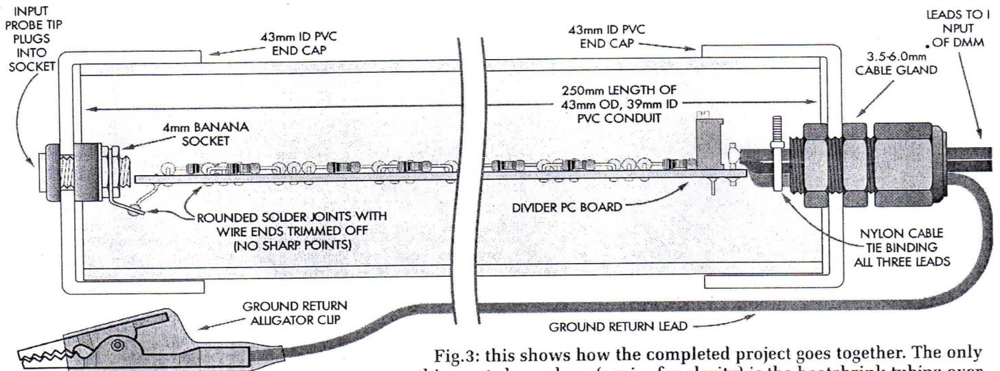
Fig.3: this shows how the completed project goes together. The only thing not shown here (again, for clarity) is the heatshrink tubing over the PC board. This provides extra electrical insulation.
