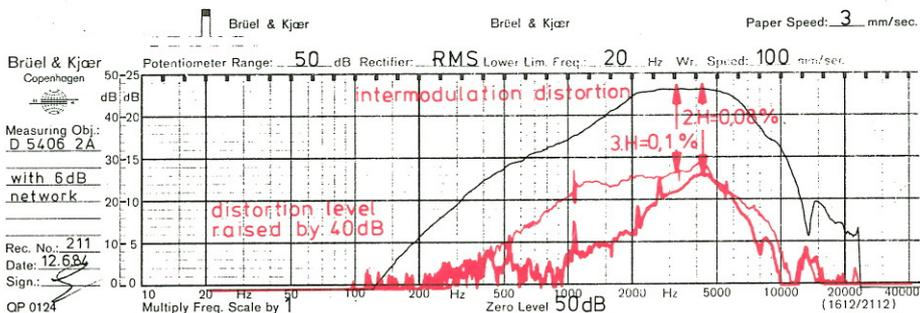
The intermodulation distortions are very low not only around 3 kHz but also at the low end.
