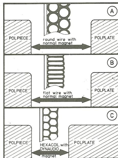
Schematic drawing: airgap of a usual magnet system with stamped pole pieces. A) with conventional V.C., B) with a flat wire V.C., picture C) shows a V.C. in hexacoil technique and precision turned pole pieces.
