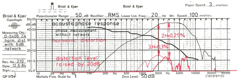
Low harmonic distortions, even at high SPL. The acoustic phase keeps smooth also beyond operating area.
