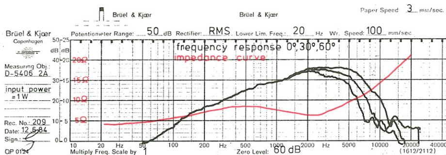
Usable from 800 Hz. Well damped resonance. No impedance peak. Off-axis curves run parallel without jumps.
