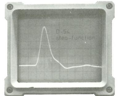
The STEP-FUNCTION of the D-54 is unusual clean. The rise indicates no break, the down slope is close to the ideal of an exponential function. No distortion or overshoot is to be noted.
