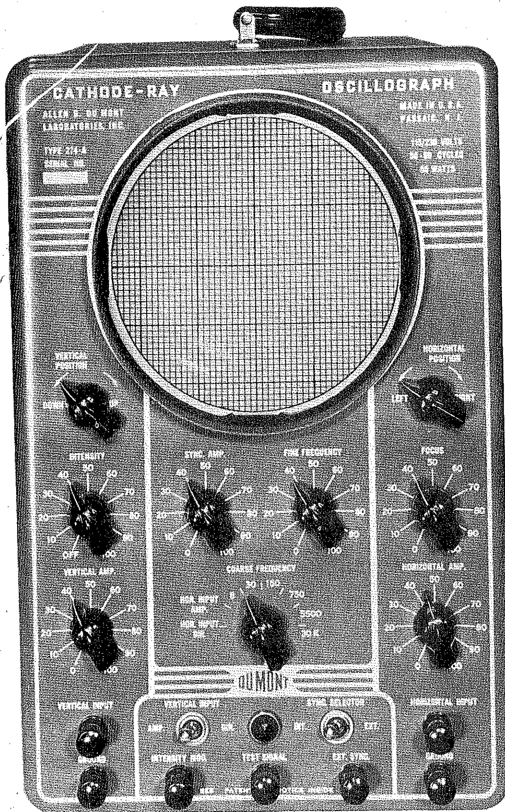
FIGURE 3-3 FRONT PANEL VIEW OF TYPE 274-A CATHODE-RAY OSCILLOGRAPH
