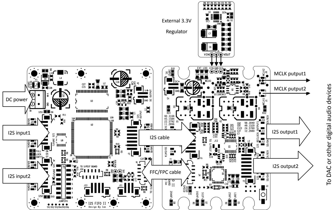
\* Please keep J5 un-connected on Dual XO II, clock board will be powered by FIFO board in this case
