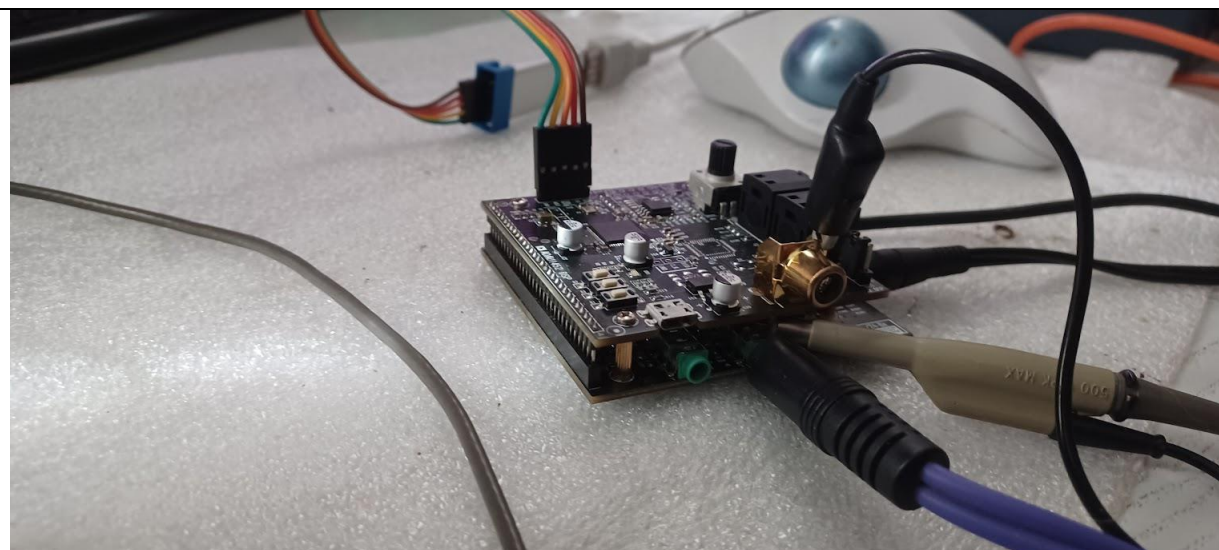
Fig. 6. DSP ADAU1452 + AD1938 under test
