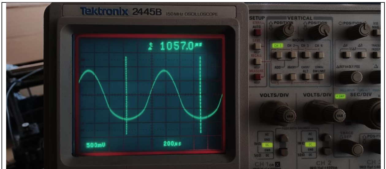
Fig. 2. Oscillogram at the DSP output which should be pure 950Hz sine wave. However, the waveform is very distorted because of high THD level. Any DSP registry settings (Fig. 8 and 9), different sampling rates etc. didn't help to fix the problem. The same THD problem is inherent in the output of all 8 DSP channels.
