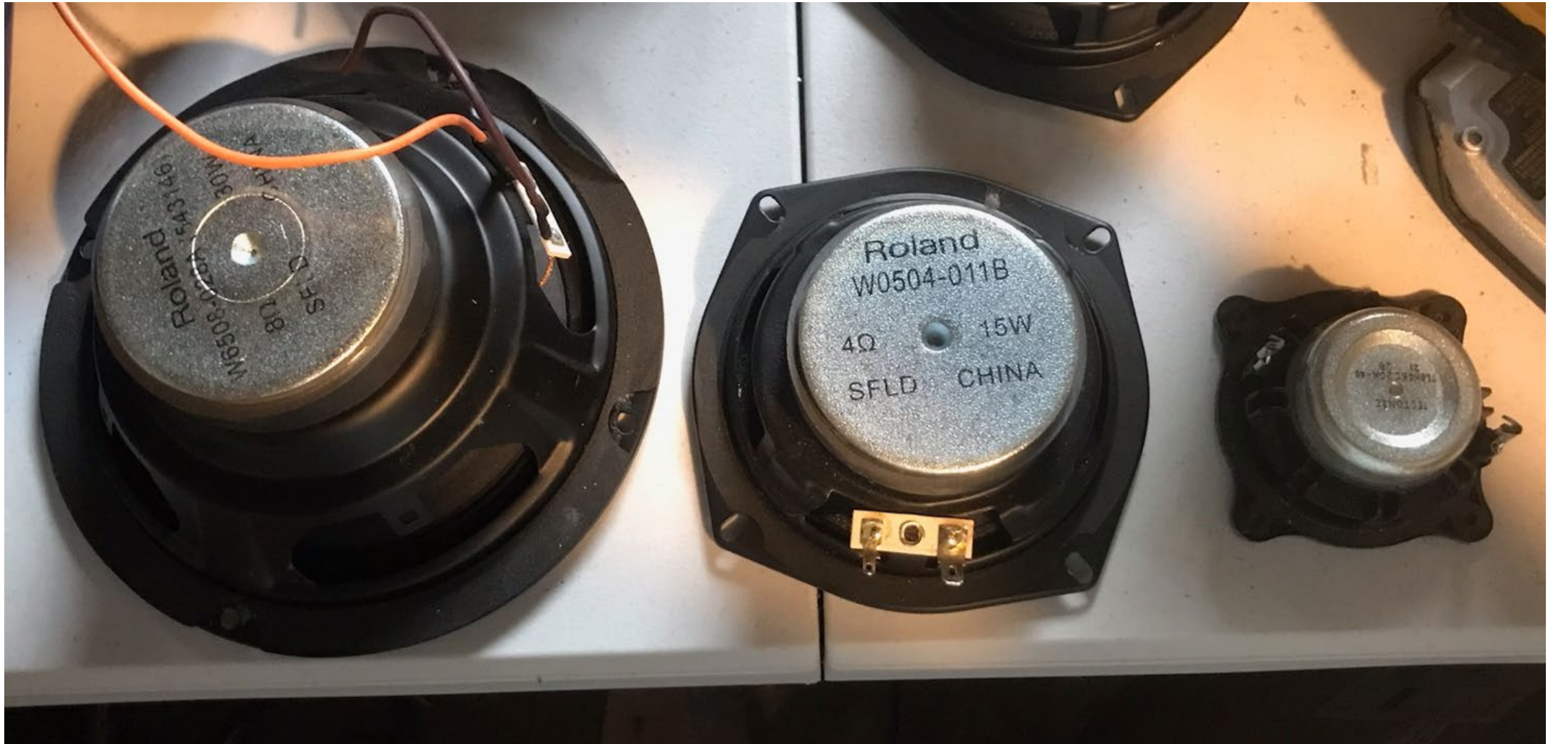
Roland 30W 8 ohm, ripped out of amp that might be used as an option, if using (4) drivers in the guitar horns.
