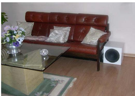
The visible part of the HideAway is only 32 x 32 x 32 cm. Although the cabinet is made by relatively thin material, it does not vibrate much. The front baffle is 22 mm MDF, and the box has a cross brace. The aperture, next to the driver, is 28 x 150 mm. There is no chuffing. Footprint is 30 x 140 cm. Stuffing is light in the box and first half of the line.
