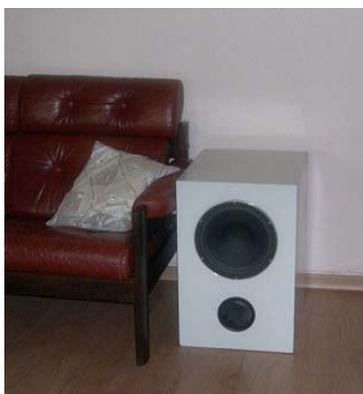
Vented box with 10" Beyma (Fs 31 Hz, Qts 0,36 and Vas 115 liters). The internal volume is 81 liters. This is big as well, and suffer from noise caused by air turbulence in the port (chuffing). The sound is "big", but I do not like the sound of a vented box.
