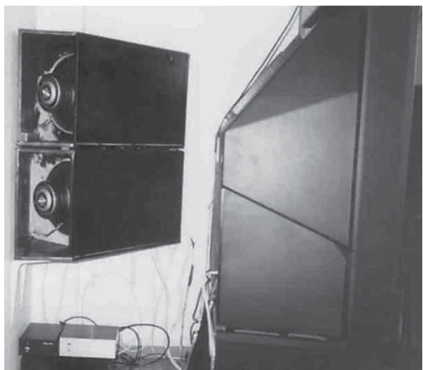
PHOTO 3: Subwoofer installed on the corner of the listening room with the equalizer and the power amplifier below.
