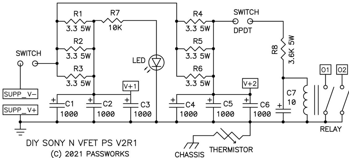
You will note the more elaborate filtering, made necessary by the VFET's exposure to rail noise and the larger thump of the circuit on turn-on/off.
