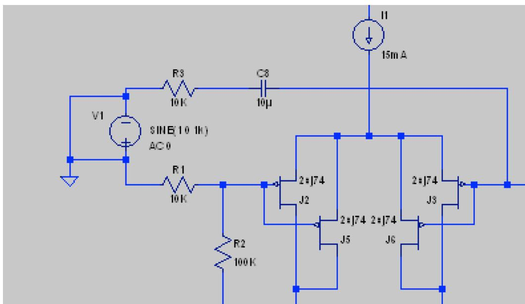
3. Inject some AC into the feedback loop:
