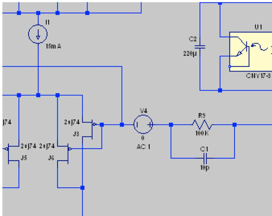
4. Run AC analysis simulations with various LTP currents. Adjust the LTP tail resistor each time to zero out the offset.
