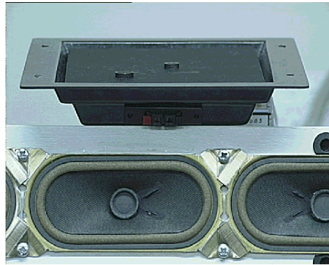
(b) The AM1-3 DML viewed from the side. Note the small overall thickness of the loudspeaker.
