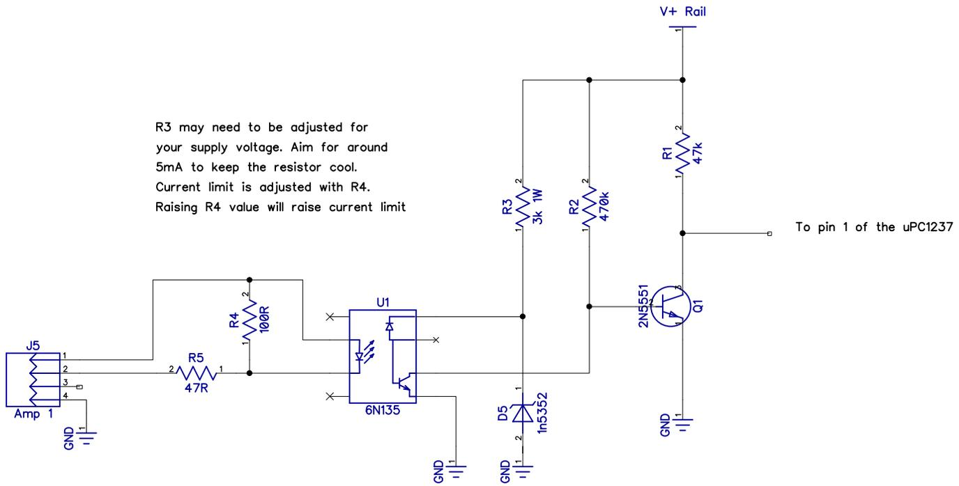
R3 may need to be adjusted for your supply voltage. Aim for around 5mA to keep the resistor cool. Current limit is adjusted with R4. Raising R4 value will raise current limit
