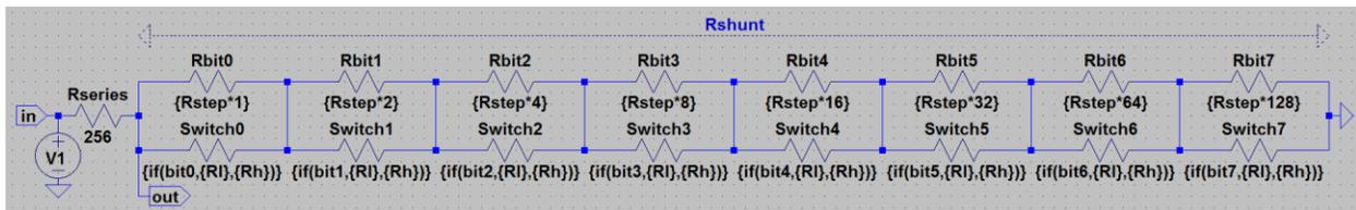
The above picture shows a ladder network that is supported by the excel sheet. The simulation file (LTspice) for this ladder network is included in the .zip-file that is made available.
