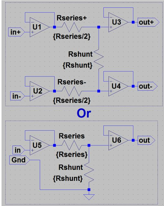
The above picture shows the configurations (among others) that can be implemented using a shunt potentiometer and a fixed-value series resistor.
