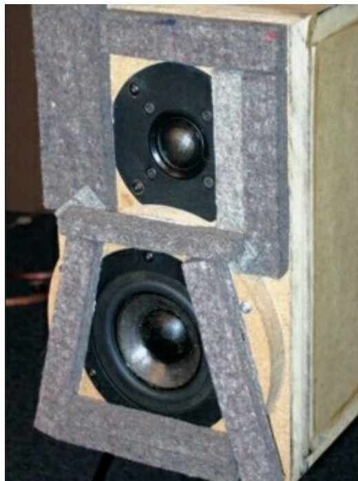
Photo 6: Baffle with full treatment of felt.
