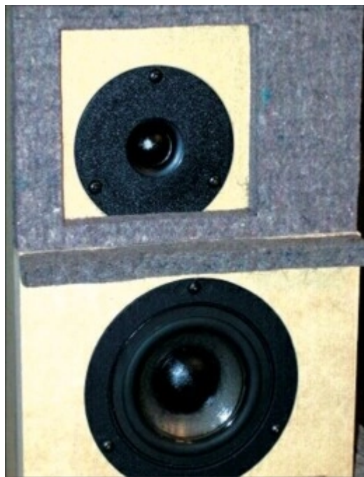
Photo 3: Adding felt block to tweeter face.
