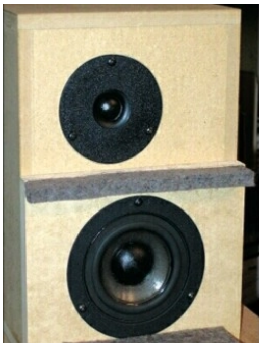
Photo 2: Felt added between drivers.
