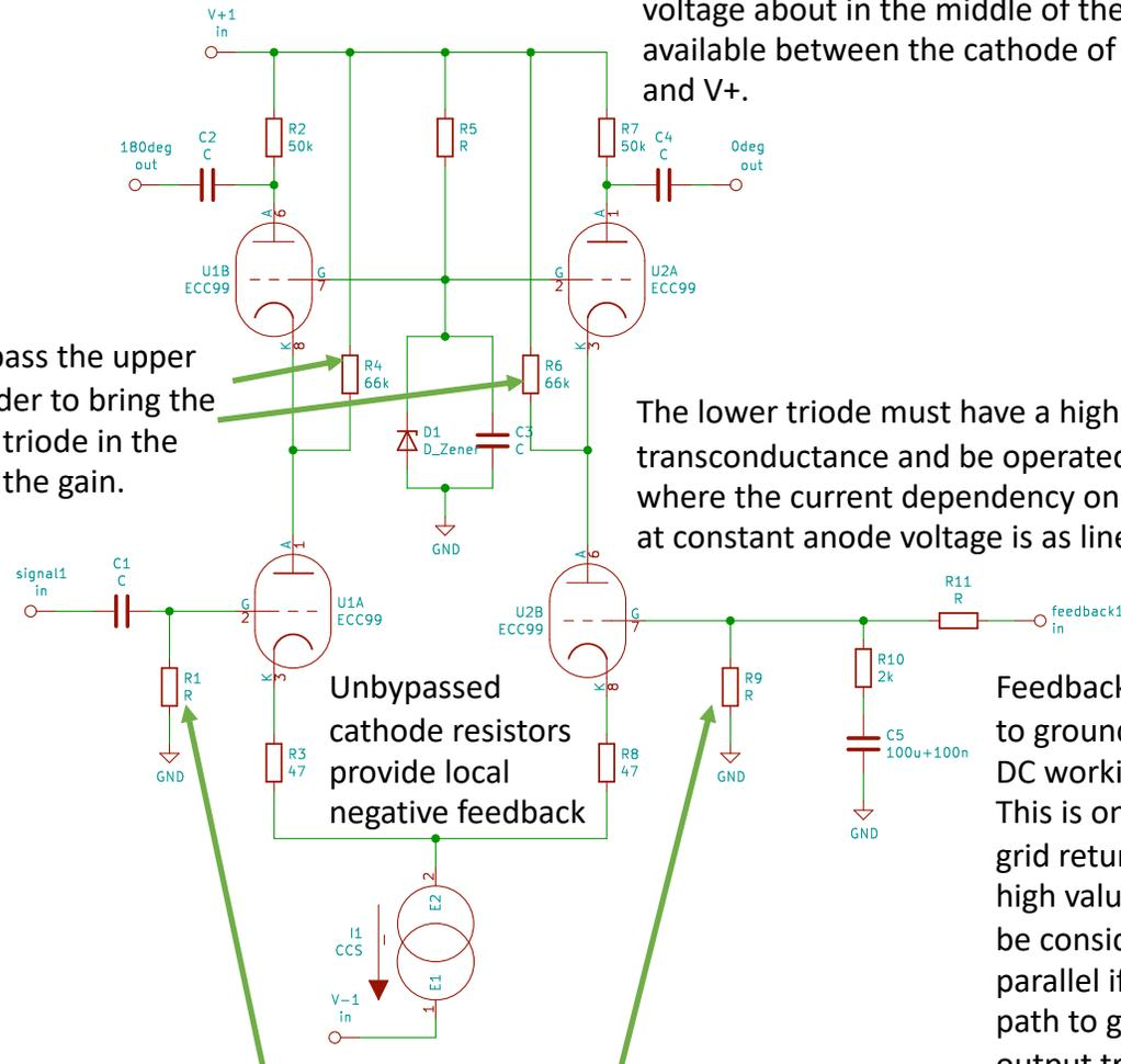
Unbypassed cathode resistors provide local negative feedback
