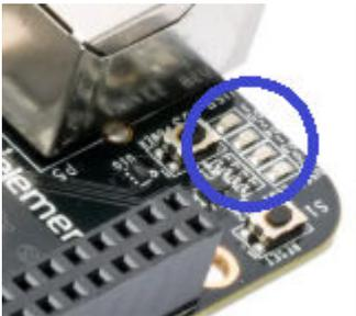
At first time booting from SD-card after 1-2 minutes the BBB should be running and connected with your LAN.
