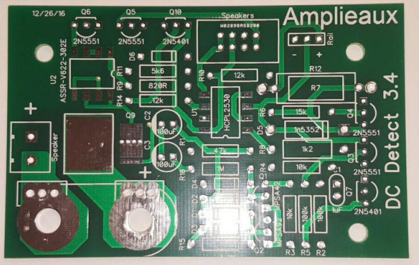
DC Detect 3.5 is a DC offset detection board with an integrated solid state speaker relay designed to mount on the power studs of a standard 3/4" center 5 way binding post assemblies. It communicates with an Amp Control board to operate. The speaker output from the amplifier is completely optically isolated from the control board to eliminate the possibility of damage to the control board, as well as eliminating the possibility of ground loops between amplifier channels.
