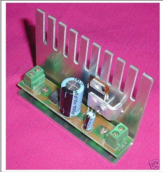
This is a complete replacement or add on regulator module for Antek power supplies. It includes a 5V LM7805, 1000uF 35V capacitor, 1A 400V bridge diode, PC board, 2 connectors, 10uF capacitor, and aluminum heatsink housing. Shipping weight about 1/4 pound.
