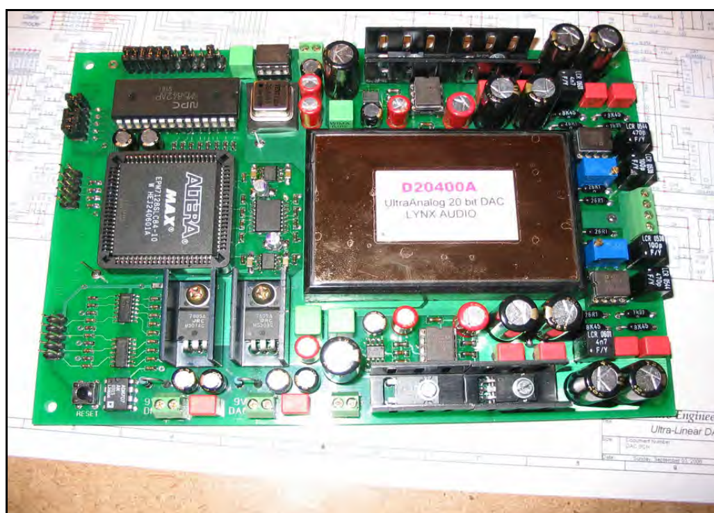
Figure: 8 Lynx30v1 DAC board layout
