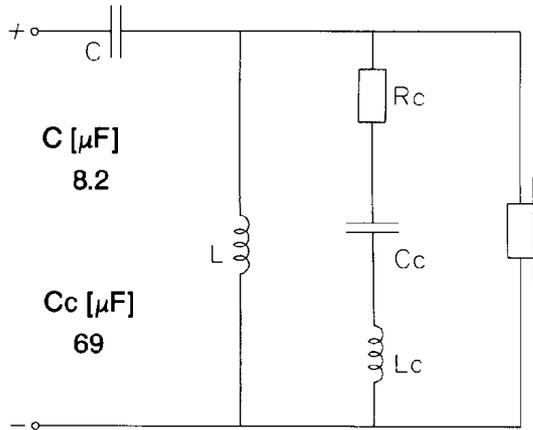
It is recommended to use at least 2<sup>nd</sup> order (12 dB/oct) cross over for this drive unit. The load provided by the cross over should be as low as possible at the tweeter resonance frequency. To ensure maximum electrical damping at resonance, and consequently minimum excursion, it is also recommended to apply the parallel compensation circuit shown. This is essential for high power input. The circuit shown is the one used for the powerhandling tests.
