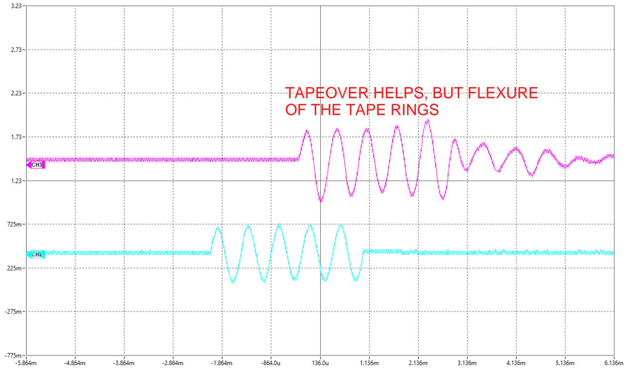
Horn has been taped over at 1596 Hz
