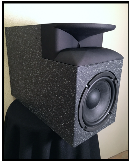
Figure 4: This is the 6" bookshelf speaker prototype that produced the data for figs. 5 & 6.
