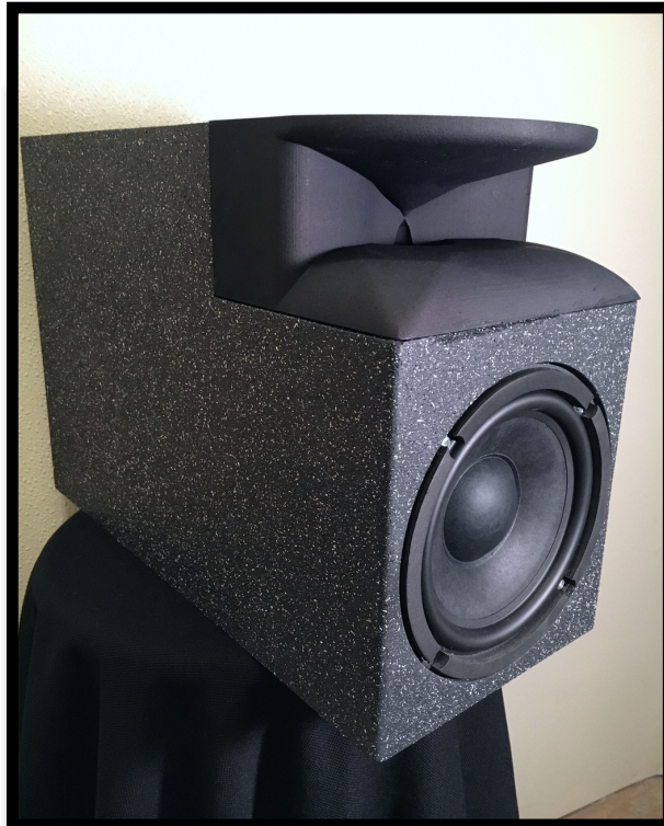
This 6" two-way concept prototype would make an outstanding consumer speaker or professional studio monitor with the right industrial design and electronics compliment.
