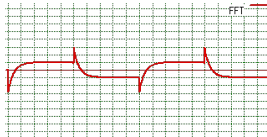
Figure 7. 400 Hz square wave reproduction.
