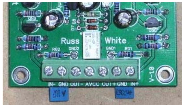
Figure 1 – RG resistors gnd pads & 4.7nF capacitors
