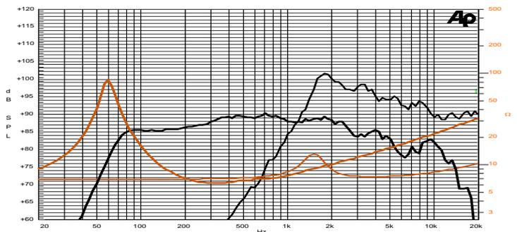
Frequency Response on 8 Lt @ 68 Hz Vented Box @ 1W, 1m
