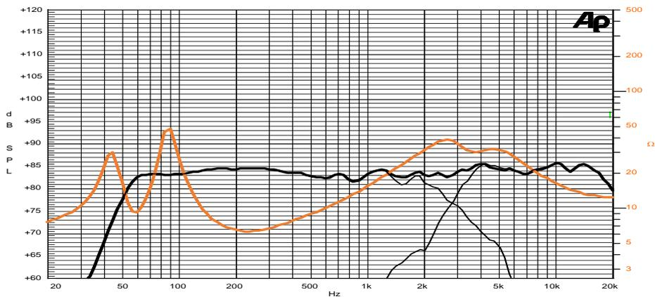
Frequency Response on 9 Lt @ 58 Hz Vented Box @ 1W, 1m
