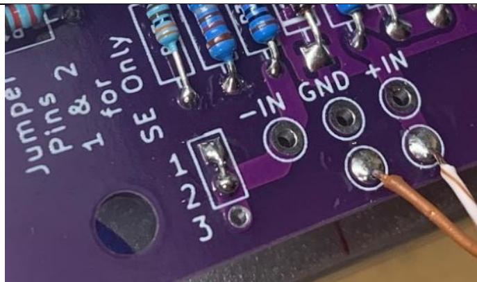
Example: Hardwire jumper installed for SE Only Hardwired SE Input
