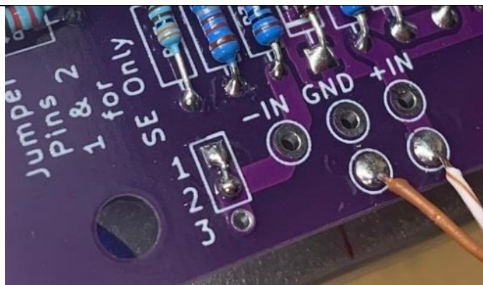
Example: Hardwire jumper installed for SE Only Hardwired SE Input
